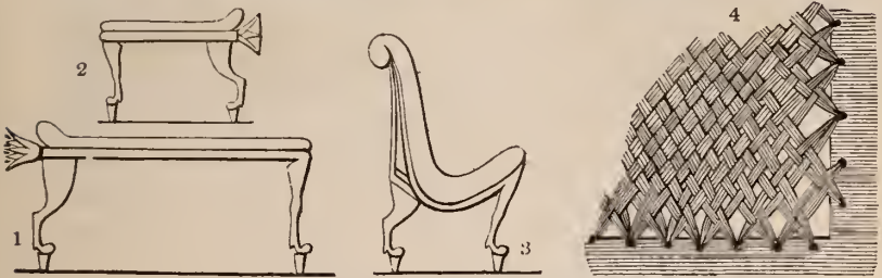
Fig. 1. A διφρος or double chair, without a back. 2. A single chair, of similar construction. 3. A kangaroo chair. 4. The seat, formed of interlaced string.
